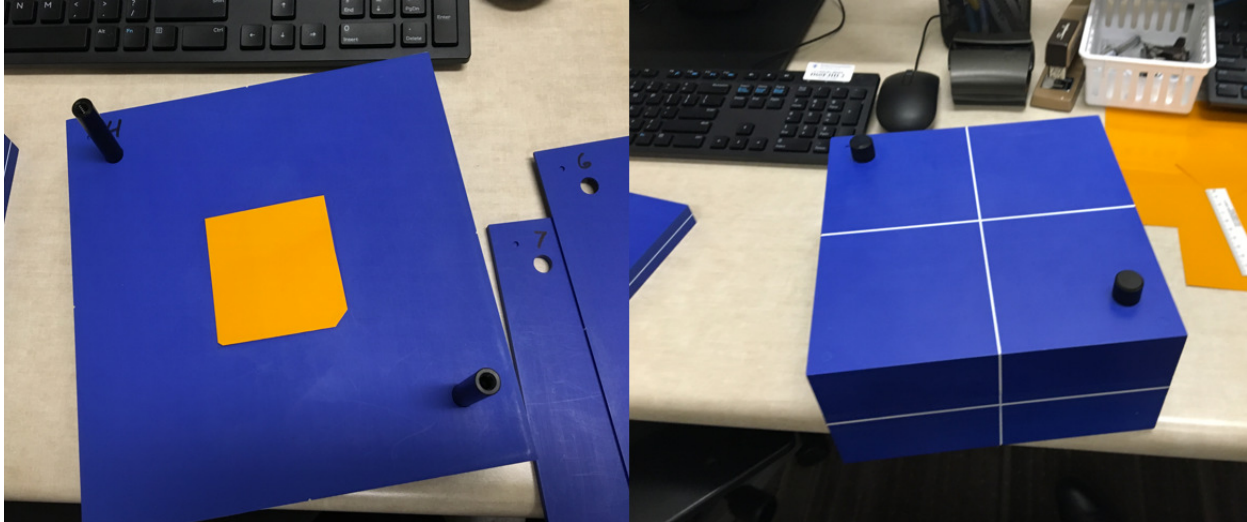
Figure 9 - LOADING THE FILM INTO THE STEREOTACTIC DOSE VERIFICATION PHANTOM
